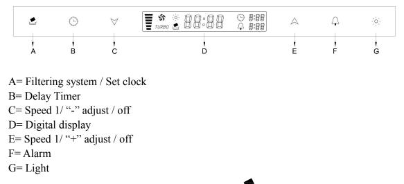
When the Key A is flashing, at the same time " is flashing on the digital display, it reminds the user to clean the filters. After it's cleaned and then assemble back, push the key A till the light is off to set the function again.
