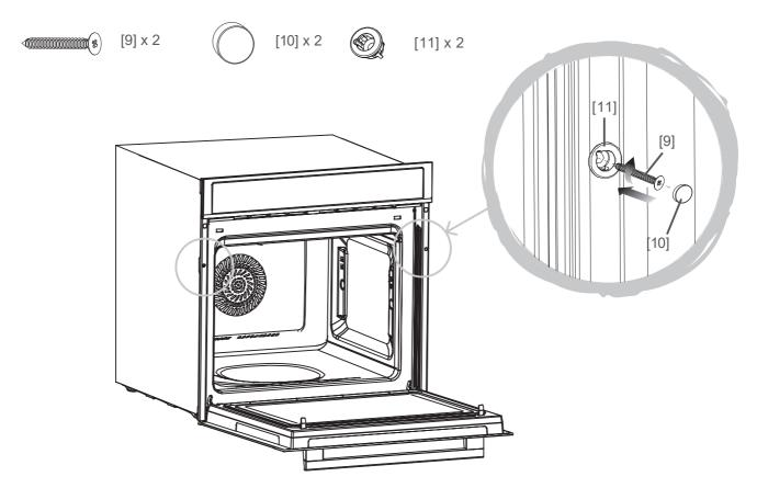
Once the oven has been lifted into place inside the appliance housing, locate the two holes in the casing of the oven and fix it into place using [08], [09] and [10].
